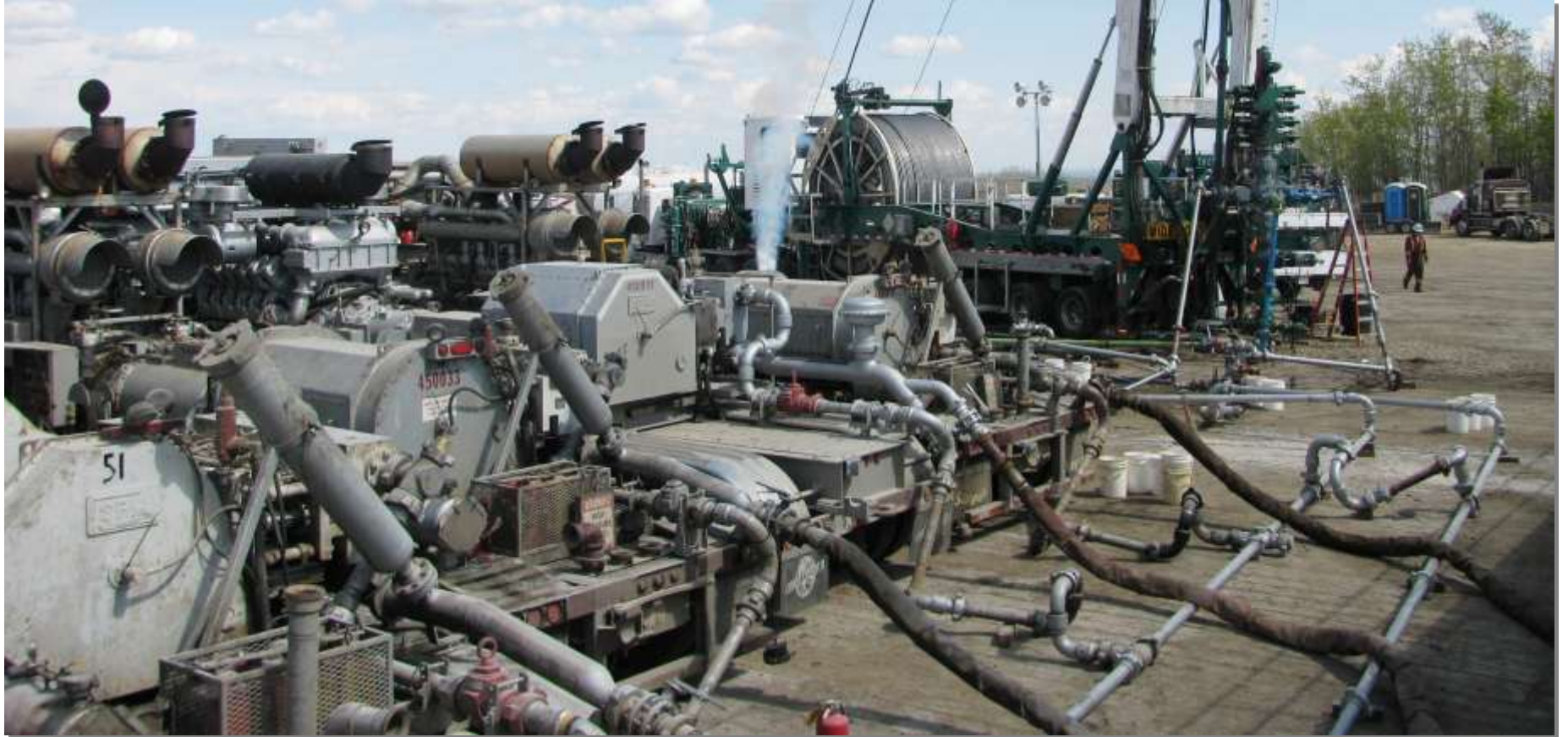
Hydraulic fracturing operation showing Weir SPM frac pumps connected via flow control products to the wellhead
